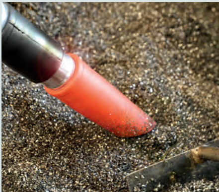
Recovery of metal chips
